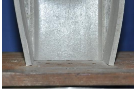
Figure 8. End of an I_3 stub tested on a direct contact condition
