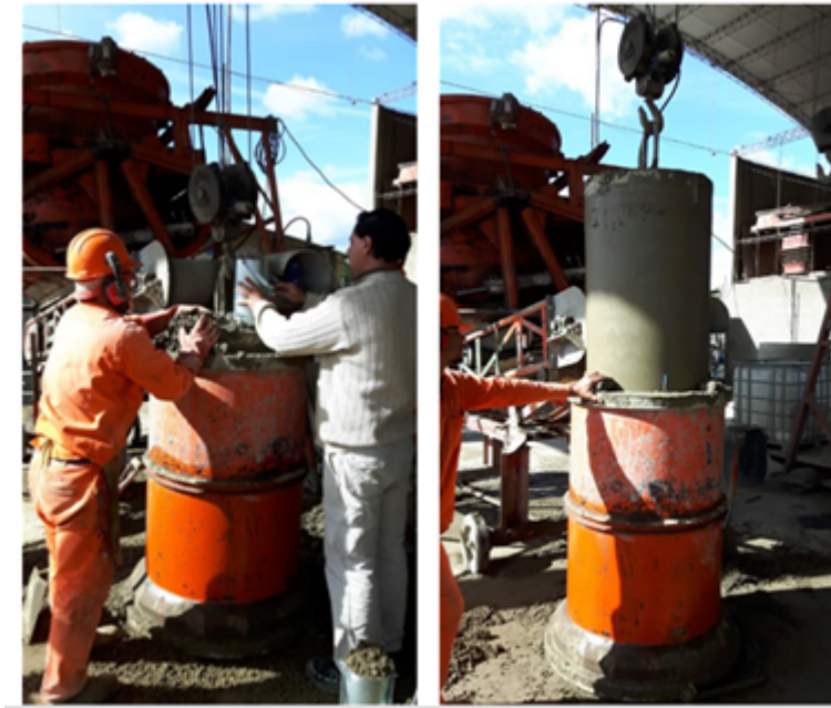
Figure 1: Molding and vibrating process. Demolding
