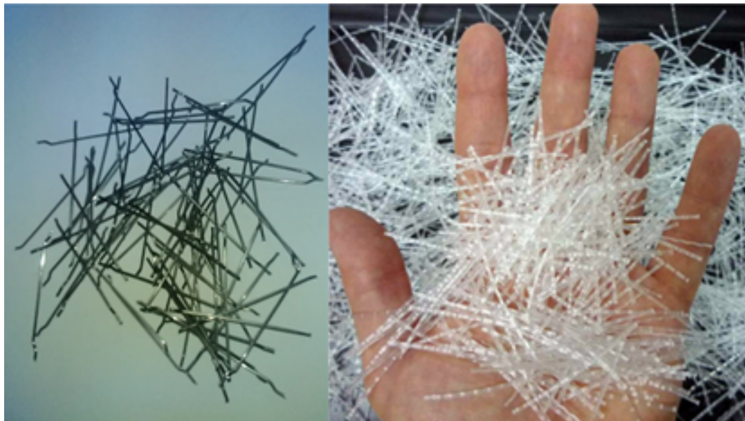
Figure 4: Steel (left) and Polypropylene (right) fibers
