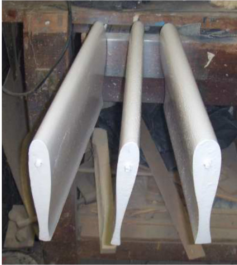
Fig. 4: LOC Schilling profiles (Lima & Fernandes, 2010; Machado et al., 2013). From left: NACA-Schilling, Slender Schilling and Blunt Schilling.
