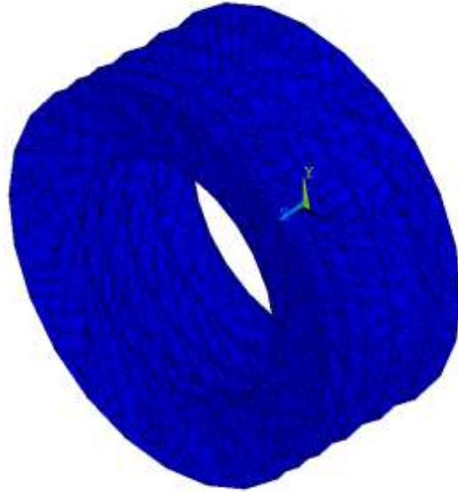
Figure 11. Vibration mode for Kresling origami structures during initial unfolding
