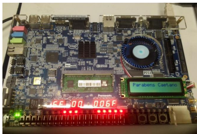
Figure 4. Development Kit Altera Cyclone IV-150 DE2i
