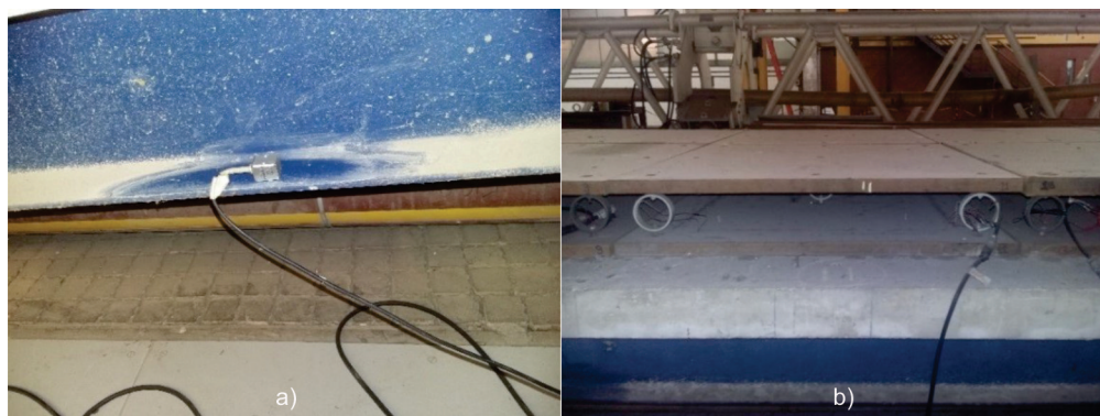
Figure 3: Sensors details: a)Accelerometer fixation; b)Force platforms
