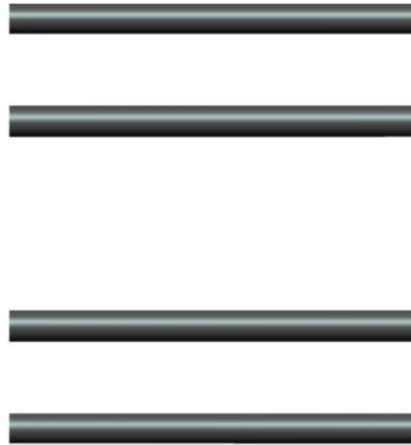
Figure 8. Optimized cell obtained by Guth (2012), by maximization the thermal conductivity in the x direction. Font: Guth (2012, p. 68).
