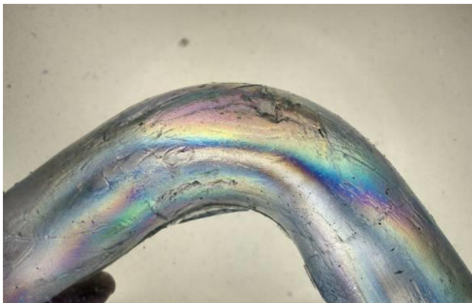
Figure 4 – Deformation curves in a resin sample
