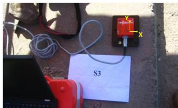
Figure 6. Accelerometers over the bridge
