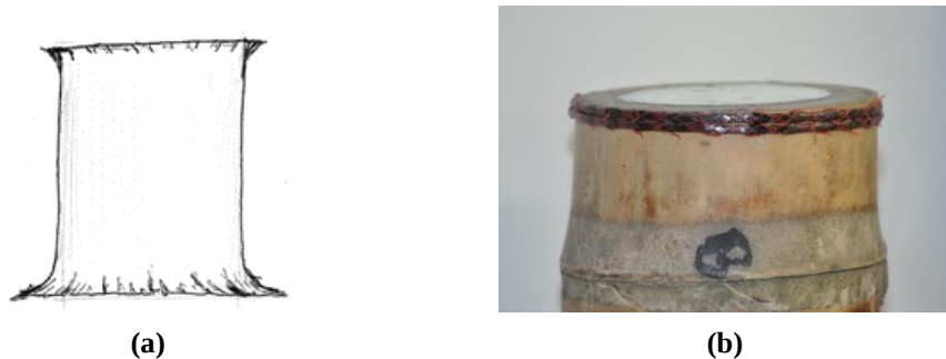
Figure 2. a) Failure by crushing of the end fibers (Quintero et al., 2016); b) Top carbon fiber stripes. After this stage, they were glued with an epoxy sticker.
