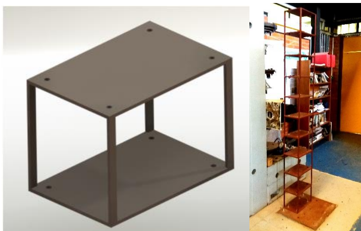
Figure 1. Steel module (left) and experimental reduced model of a tall building assembled (right)
