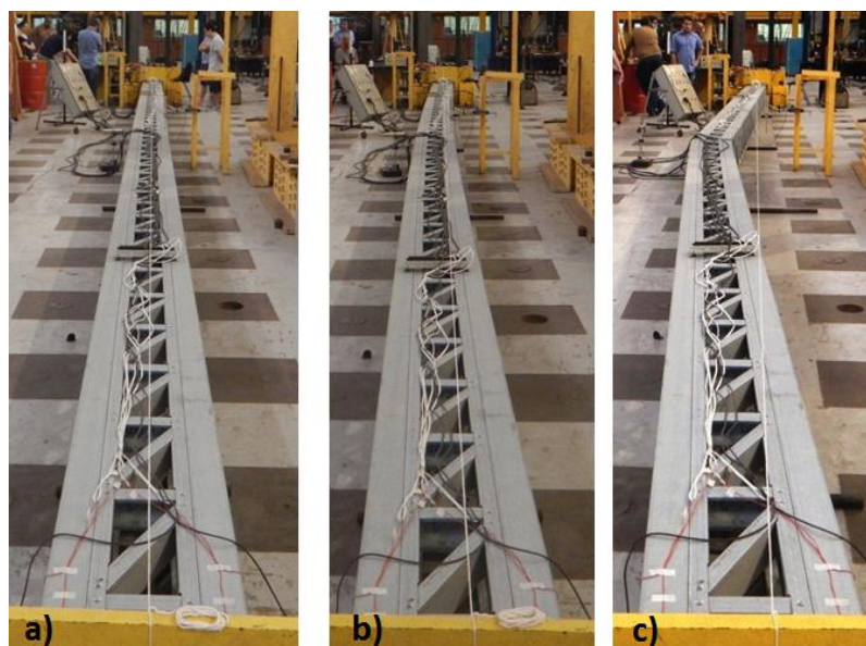
Figure 9 - Global buckling of laced built-up column 16m long. (a) Starting the test (low compression load). (b) Close to the collapse load. (c) After collapse.
