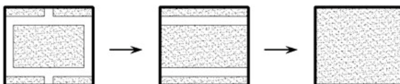
Figure 14 - Method of homogenization of masonry
