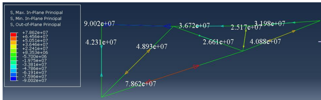
Figure 14: results of the simulation with the final truss' topology simulated with Abaqus.
