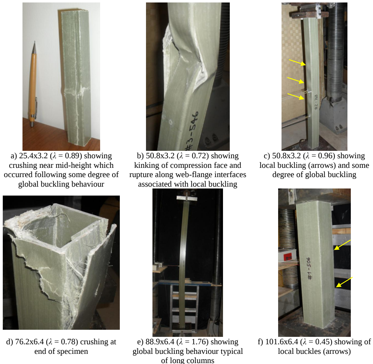
Figure 11. Representative failure modes of column specimens.
