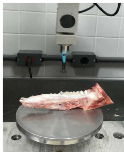
Figure 2. Assembly scheme for the compression test by EMIC
