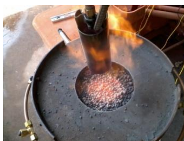
Figure 2- Combustion Ignition of the solid fuel in the combustion cell
