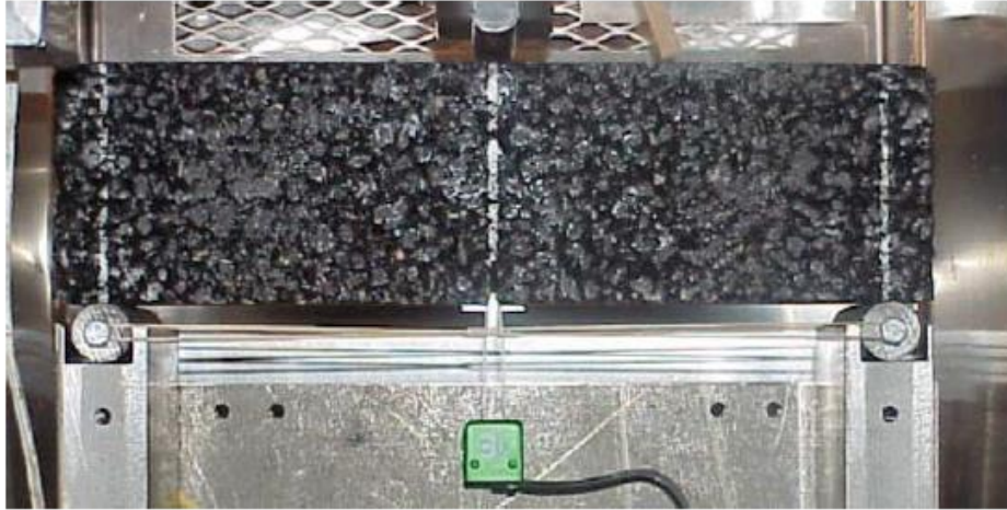
Figure 2: SE(B) test fixture and clip gage (Wagoner et al., 2005).
