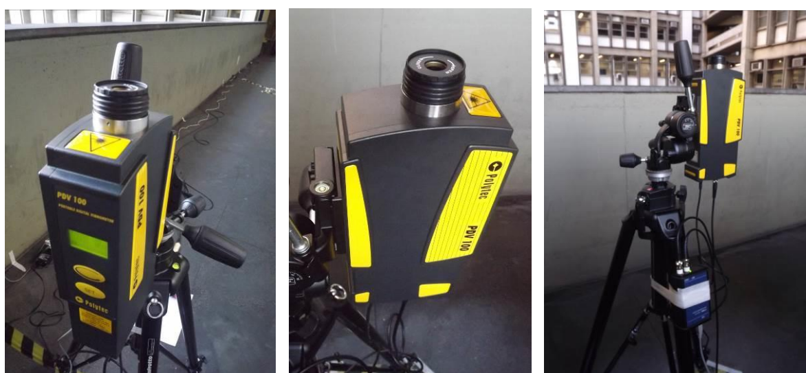
Figura 10. Vibrômetro à laser Polytec (Portable Digital Vibrometer: PDV-100)
