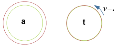
Figure 3. Axis-symmetric (a) and torsion (t) deformation modes
