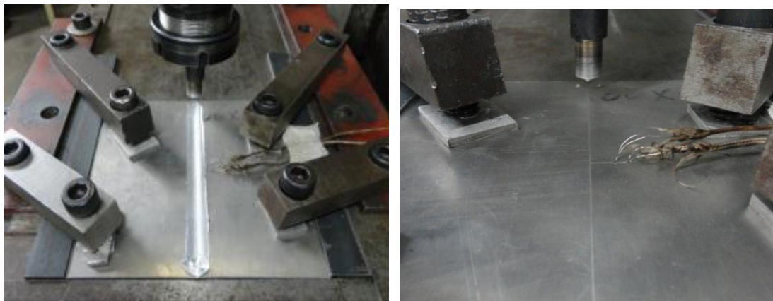
Figure 1. a. Friction stir welding (FSW) device and mounting, b. TC's locations
