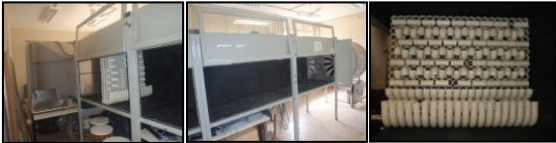
Figure 1. Wind tunnel and turbulence generating panel at LaCAF-FEC-UNICAMP
