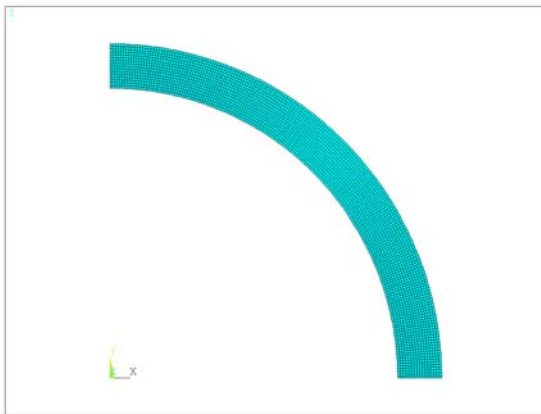
Figure 6 – Solid FE mesh of the pipe LT15.0 without ovalization
