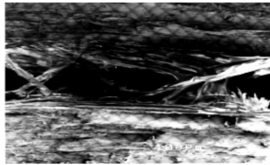
Figure 3. Fibre bridging mechanisms at the FPZ of wood: Vasic & Smith (2002)
