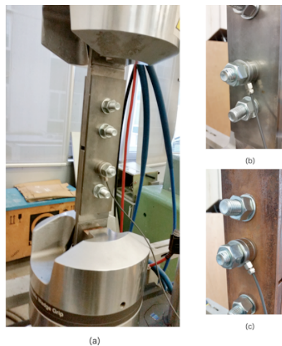
Figure 4. (a) Experimental set-up for the test; (b) S235J steel joint; (c) COR-TEN steel joint.
