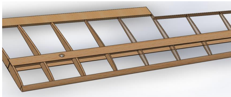
Figure 2. CAD damaged wing model with hole near the binding spot.
