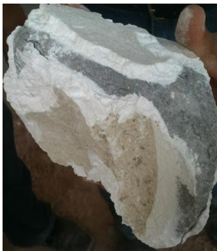
Figure 2. Shoddy product originated by lack of control of the parameters of the lime kiln.
