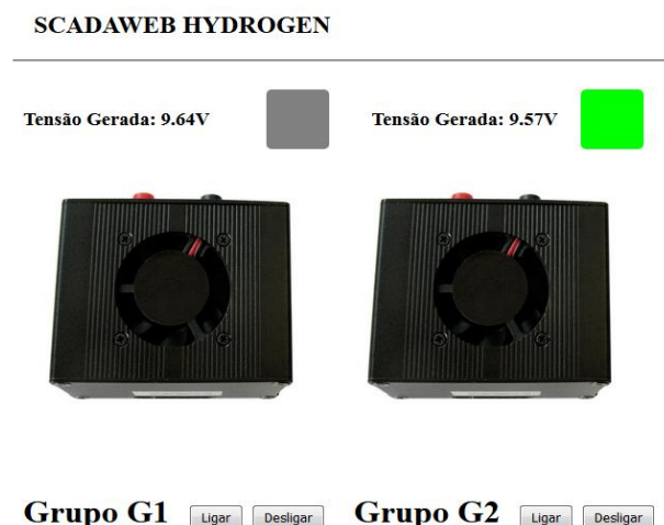
Fig. 2. Layout do supervisorio SCADAWEB Hydrogen.
