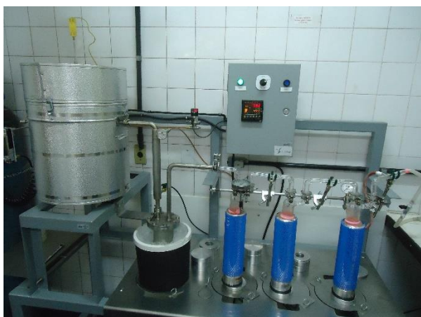
Figure 1- Experimental Setup of the vacuum pyrolysis experiments, showing heating chamber to the left, one metallic trap, 3 glass traps to the front and the control panel to the back
