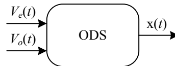
Figure 4: ODS composed of two inputs, P = 2 (torque, V_e(t) , and inclination angle, V_o(t) ), and one output, H = 1 (velocity of the vehicle in a longitudinal direction, x(t) ).
