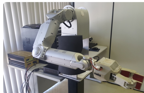
Figure 1: Meka Robotics A2 Arm at LARA
