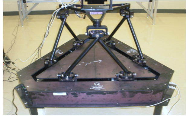
Figure 1: 6 DOF platform used for system disturbances.
