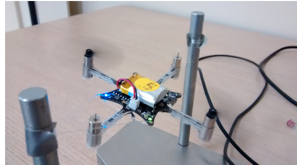
Figure 9: Crazyflie tied between two columns for pitch control test.
