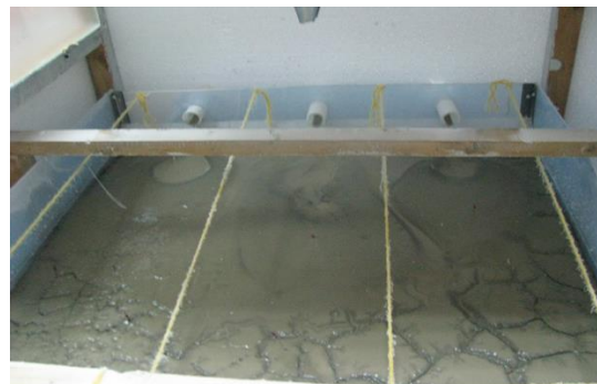
Figure 6. General view of the inwashed beach at the temperature of -45 °C .
