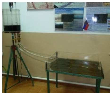
Figure 3. General view of the laboratory-scale plant for the inwash technology modeling (Patent RU 122098)
