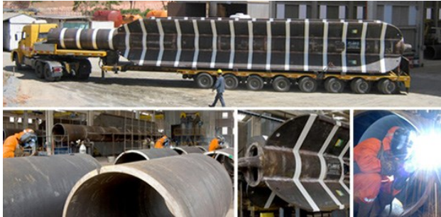
Figure 1. Torpedo pile T-120 tons (Fluke Subsea, 2016).
